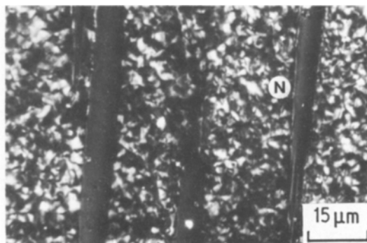
Figure 16 Optical micrograph of HMU fibres in matrix carbon from D112 coal extract; 0.6 MPa.
