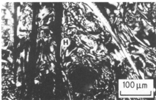
Figure 10 Optical micrograph of CVD coated fibres in matrix carbon from A240 pitch; atmospheric.
